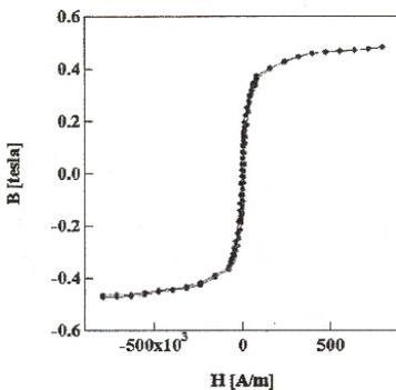
CM-10-10 showing paramagnetic characteristics
