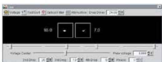
Initial Drop Delay Profile with Spherotech Drop Delay Calibration Particles
